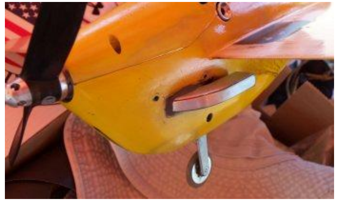
Two Differing approaches to the FAI mandated covered exhaust requirement. Alex Tupenov's design (above), and Dick Lambert's rendition (Below).
