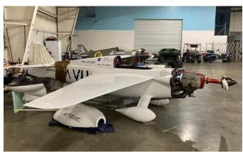
"Déjà vu" with cowling removed showing prop extension and Exhaust routing.
