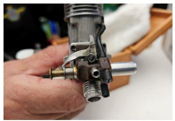
This engine incorporates a rear drum valve with (I think) at least a 5 function shut-off valve).
