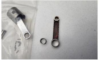
One version of this engine used a needle bearing connecting rod. I understand, the bearing roller cage is one of the more difficult/delicate parts to make. I don't know if the roller bearing rod was worth all the extra effort compared to the regular type of rod.
