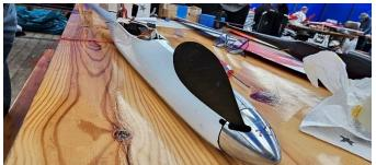
I have to admit I wouldn't normally give this thin (250 Euro) paddle blade prop a second look. That is until I saw it perform on the Czech world champions racer. Then all doubt was removed and I can see why it commands its price. Not apparent is this prop needs to swing forward & aft to extend the life of the engine bearings. Who would have thought?
