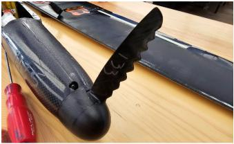
How about this left handed shark tooth racing prop. From the ingenious minds in Australia, this saw toothed single blade prop (for spanwise flow straightening) with 133mm of pitch. Big Bruce DeChastel claims it's much faster in good hot weather & slower in cool wet weather. Why the difference is still to be determined... It might be harder to hand flip though...
