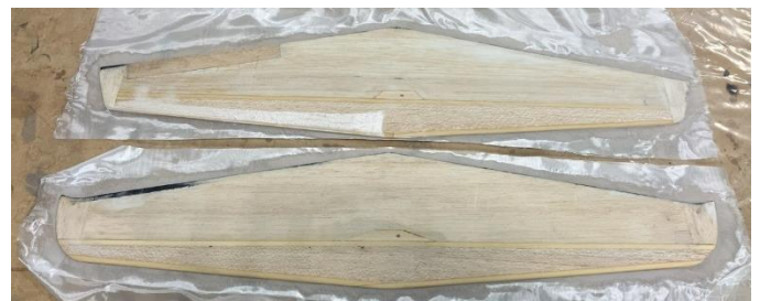
(Top), Gerry's new Sport Goodyear Models assembled and awaiting paint. (Middle and bottom), showing the Vacuum bagged fuselages and wings.
